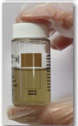
Look through the bottle Viewing Window. Compare the Test Solution color to the Test Standard printed above the Viewing Window.
