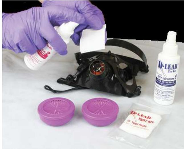
When the respirators are dry, inspect all of the valves, straps, face seal, and replace parts in accordance with manufacturer's recommendations.
