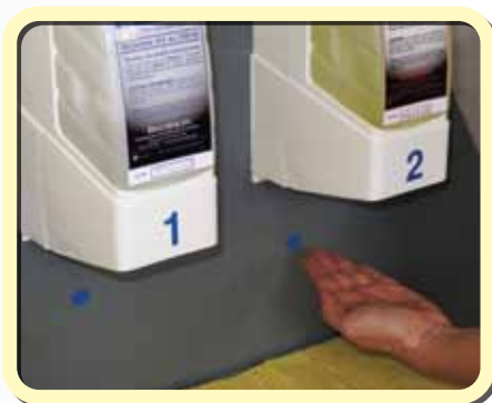
Move hand towards dot to dispense solution 2 on to hand.
