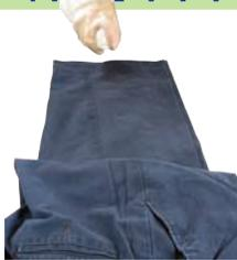
Spray the fabric above the test pad with Solution 1 until the testing area is wet
