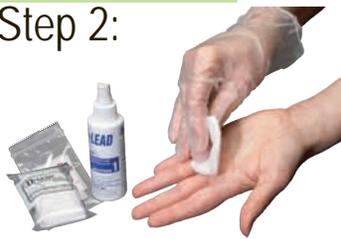
Wipe the hand or surface to be tested with the test pad
