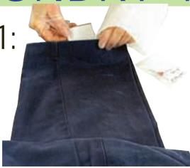
Place a test pad under one layer of the fabric to be tested
