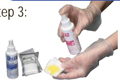
Spray the same side of the test pad 1 - 2 times with Solution 2
