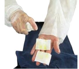
Remove test pads from both above and below the fabric and spray with Solution 2
