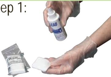
Spray one entire side of a test pad with Solution 1 until the pad is wet
