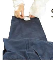
Place a second test pad on the fabric, directly above the first pad and press down firmly
